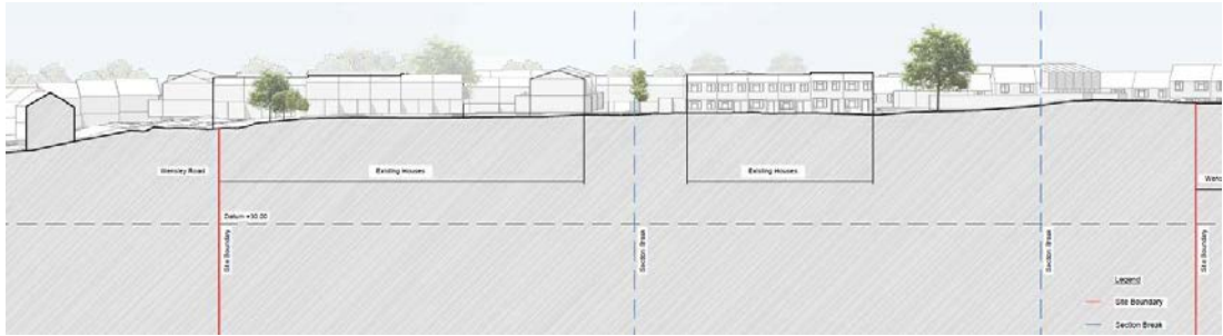
Existing and Proposed Section AA - north-south mews looking west showing Block A
