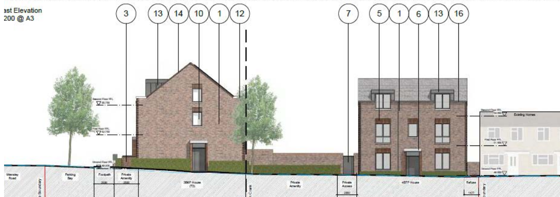
Side elevations of the Block A terrace & front elevations of the detached dwellings
