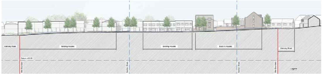
Existing and Proposed Section AA - north-south mews looking west showing Block A
