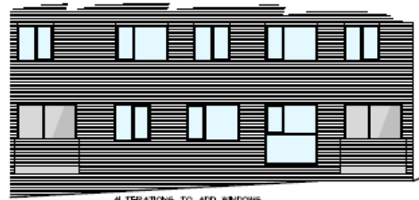
WEST/REAR PART PROPOSED ELEVATIONS (1:100)
